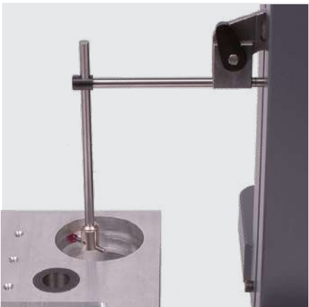
Internal groove measurement with accessories 930-2108, 930-2110 and 905-2207
