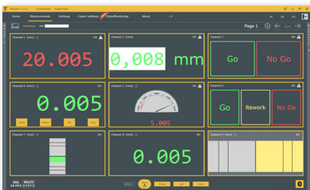
Multiple displays: Bar graph, numeric, Go/no Go and histogram for clear display of measurements
