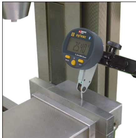
Checking the alignment on milling machine.
